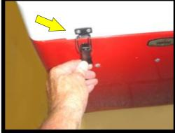
02 Open rear latches of the cover, and remove it, placing it down carefully. Repeat when reloading.
