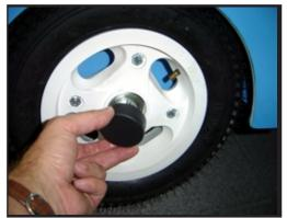
**08**With the wheel properly mounted and counterlocking pin to put the finishing cap.
