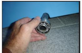
**04**Manually slide the first bearing to the end.
