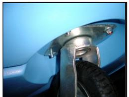
**02**Tighten the nuts with a 13mm and put the cart back on the floor.
