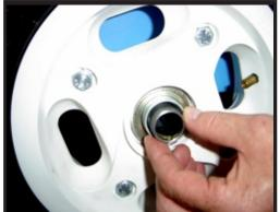
**06**With the wheel fitted, slide the second bearing and then ring back.
